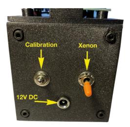
Your light module is ready to use, you have to supply it with 12V on the female plug at the back of the box, respecting the polarity (positive in the center of the plug). The left switch controls the calibration lamp, the right switch controls the 4 Xenon lamps.
