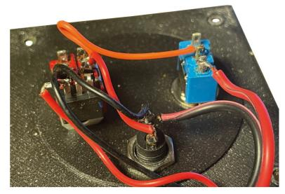
Fix the 2 switches and the 12V socket on the back cover of the light module. Proceed with the wiring using the electrical diagram on page 7. The LM 7812 voltage regulator is soldered directly to the switch (pin 1 and 2).
