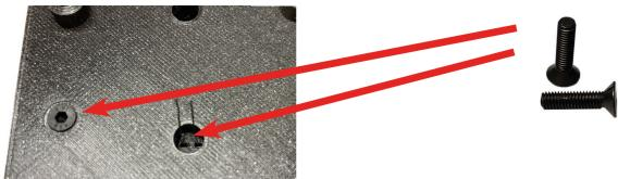
Fix on the top of the main block the lower part of the high voltage power supply box with 2 M3 countersunk head screws of 10mm length, making sure that the 2 wires of the firefly pass well in the hole provided for this purpose.
