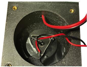
On the support of the 4 Xenon bulb sockets, connect the sockets in series as shown in the picture and insert the support in the main block. In order to maintain this support in place, you can use electrician's tape to apply the support to the bottom of the main block.
