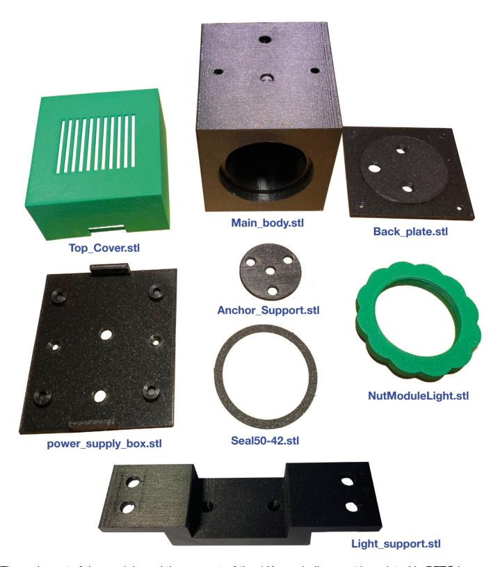
The main part of the module and the support of the 4 Xenon bulbs must be printed in PETG because the Xenon bulbs give off some heat, PETG melts at a higher temperature than PLA. The other parts can be printed either in PETG or PLA.
