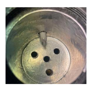
In the main block, insert the 2 wires of the firefly in the holes provided. The 2 wires will have to be covered with a heat-shrinkable sheath to avoid any short circuit.
