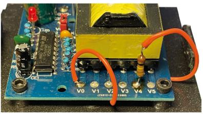
Extend the 2 wires of the firefly that we will cover with a heat-shrinkable sleeve. Then solder the 100  $K\Omega$  resistor on the converter at the V4 location as shown in the picture, and solder the 2 wires coming from the firefly (at V0 and on the other end of the resistor).
