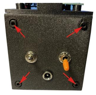
Screw the rear cover onto the main block with 4 x M3 screws of 8 mm length.
