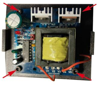
It is also necessary to solder 2 cables to supply 12V to the voltage converter. Solder a cable on the GND slot and another on the VCC +12V slot as shown in the picture and pass the cable through the hole in the box. Then fix the module in its place with 4 screws M3 of 4 mm length. On the module I used, I could not fix the 4th screw because of the heat sink of one of the transistors.
