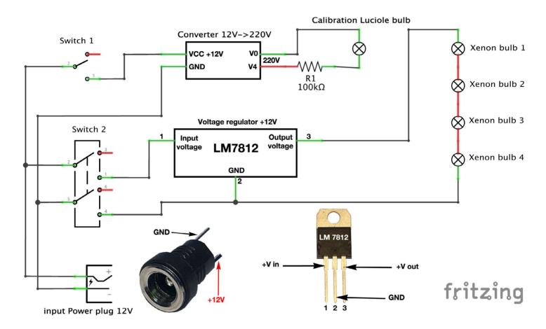
The Xenon lamps have a nominal voltage of 3V, hence the assembly in series of 4 bulbs to be able to operate under 12V. The LM 7812 voltage regulator is used here rather as a voltage limiter in order not to have a voltage higher than 12V in the Xenon lamps (the 12V power supplies tend to deliver a slightly higher voltage and the Xenon bulbs do not tolerate too much overvoltage).
