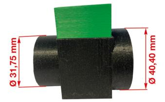
• <u>The cover</u>: To be realized in 3D printing with the file liquidCell#2.stl in PETG or PLA in the color of your choice. This cover prevents ambient light from affecting the measurement of the sample. It covers the test tube.
