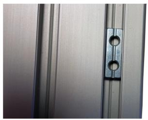
It is necessary to insert the slides in the external rails of the optical bench by using a screwdriver or key alen to position it well in the rail.
